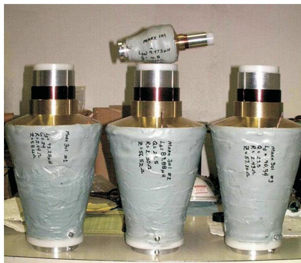
Fig. 4. TAMU Mark 101 and 301 tapered stator generators.
