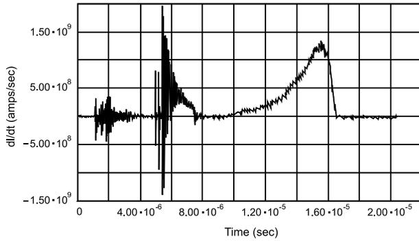
Fig. 7. The time derivative of the current for the Mark III Test #4 is shown.
