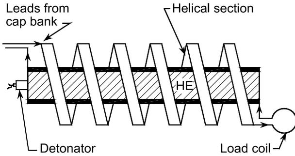
Fig. 1. The helical FCG, before HE initiation, has a cylindrical armature and a solenoidal stator, which provides much larger initial inductance than other geometry FCGs.
