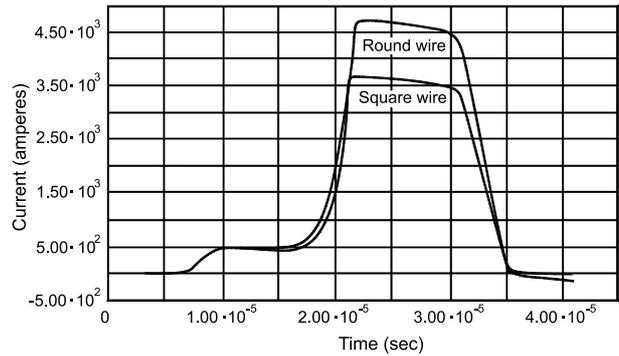
Fig. 5. Current traces from two Mark 101 tests show directly the differences in gain for round and square wire.
