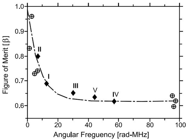
Fig. 2. Dependence of the figure of merit on the contact point's angular frequency for FCGs with constant diameter armature and single stage design. Data points are calculated from experimental data in references [Gov79], [Leh99], [Nov95], [Fow89], [Jon79], [Fre79], circle symbols, and own tests, diamond symbols. The solid line serves as guide for the eye only. Indicated are the authors' [Neu01] generators: TTU I
