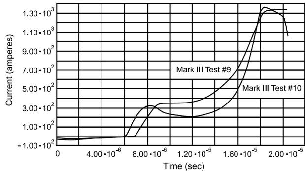
Fig. 6. The two current traces for the Mark III Test #9 and Mark III Test #10 are shown.
