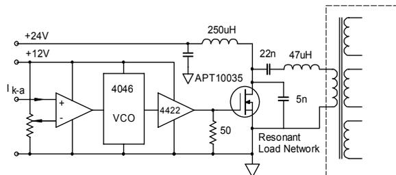
Figure 7. The Class-E power converter
