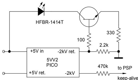
Figure 6. The keep-alive current sense circuit
