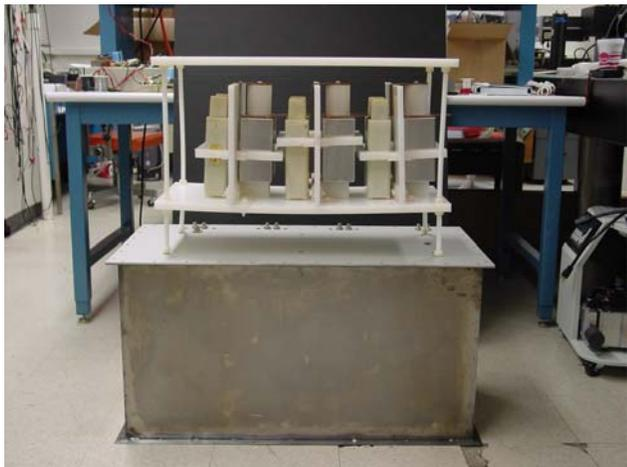
Figure 4. The Marx bank and its components
