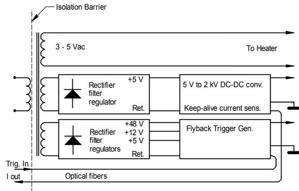
**Figure 3.** Block diagram of the floating housekeeping system
