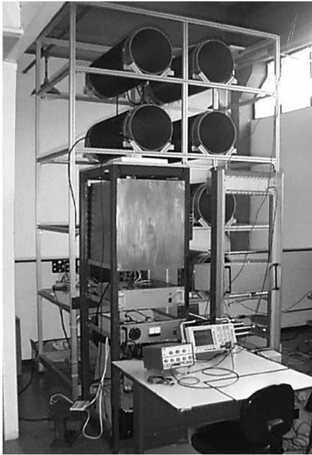
Fig. 4. Whole Blumlein system with the coaxial winding structure in the back.
