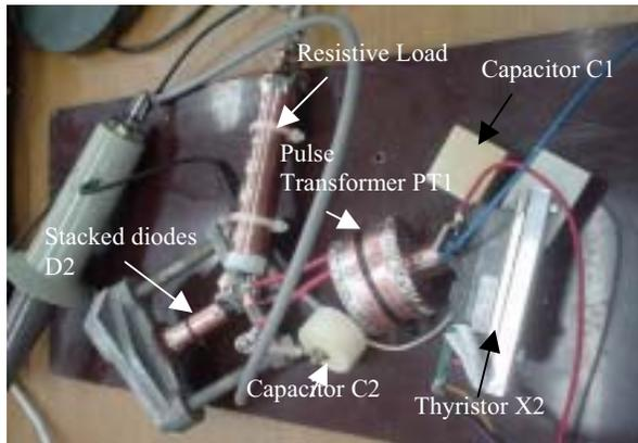
Figure 6. The experimental system of the proposed system
