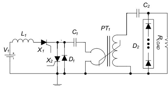
Figure 1. The simplified electrical scheme of the proposed pulse generator
