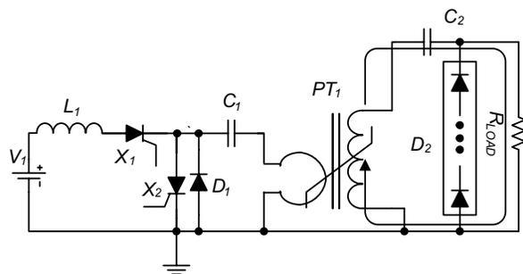
Figure 5. Output power delivery mode
