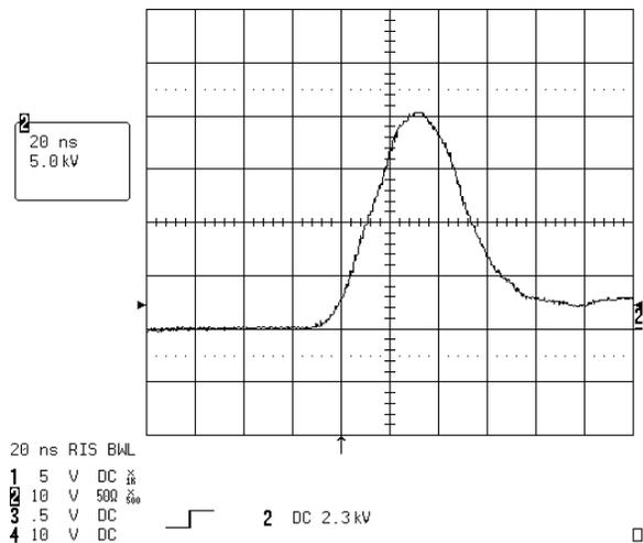
Fig. 6. Output Voltage Waveforms(5kV/div)
