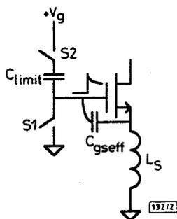
Fig. 2 Simplified schematic diagram of gate driver circuitry
