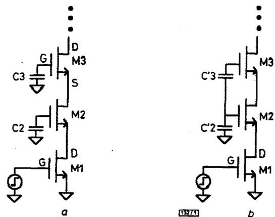
Fig. 1 Simplified schematic diagram for series operation of power MOSFETs and alternative method for series operation of power MOSFETs
