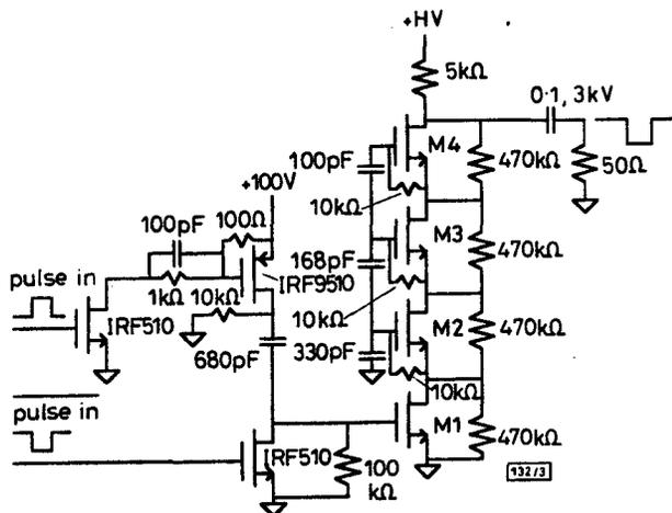
Fig. 3 Schematic diagram of 1500V pulse generator designed using the techniques presented
