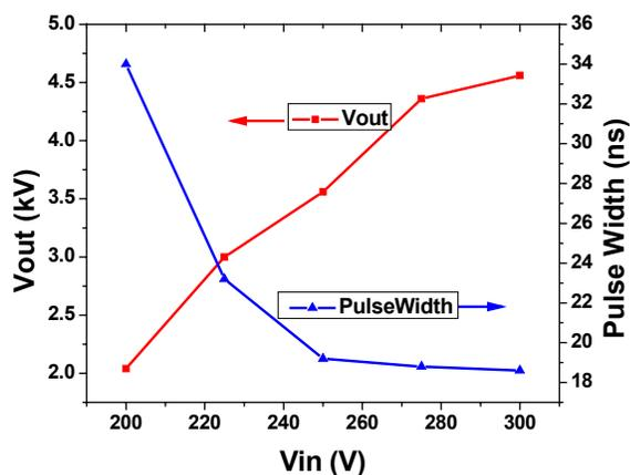
**Figure 5.** Output pulse amplitude and width vs different charging voltage
