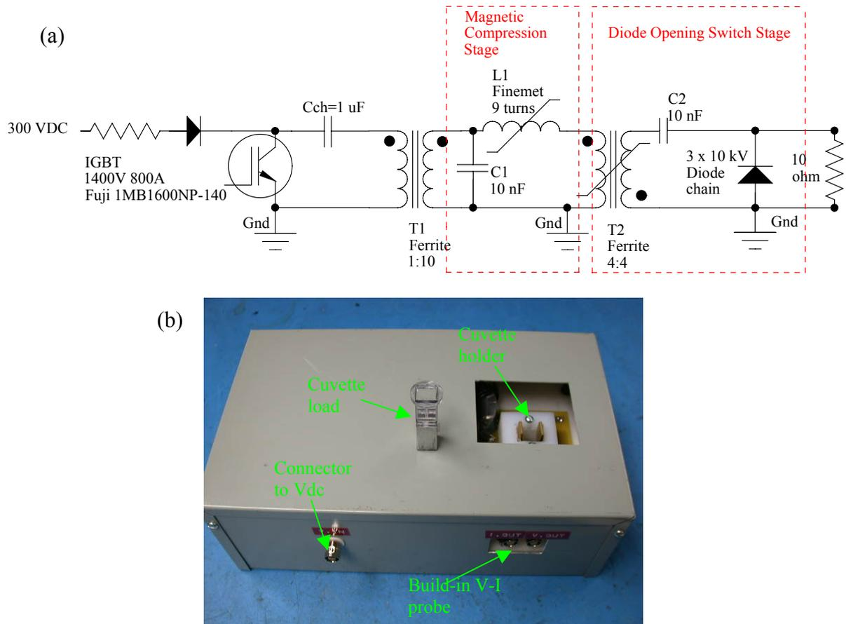
**Figure 1.** (a) Circuit diagram of the pulse generator. (b) Constructed pulse generator with a cuvette load.
