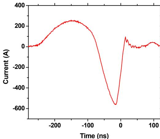
Figure 2. Current through diode D. Forward current: 256 A, 182 ns; Reverse current: 560 A, 58 ns.
