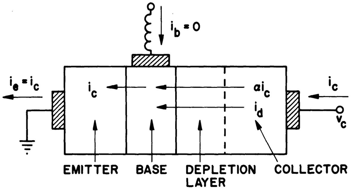
Fig. 1. Basic transit-time diode
