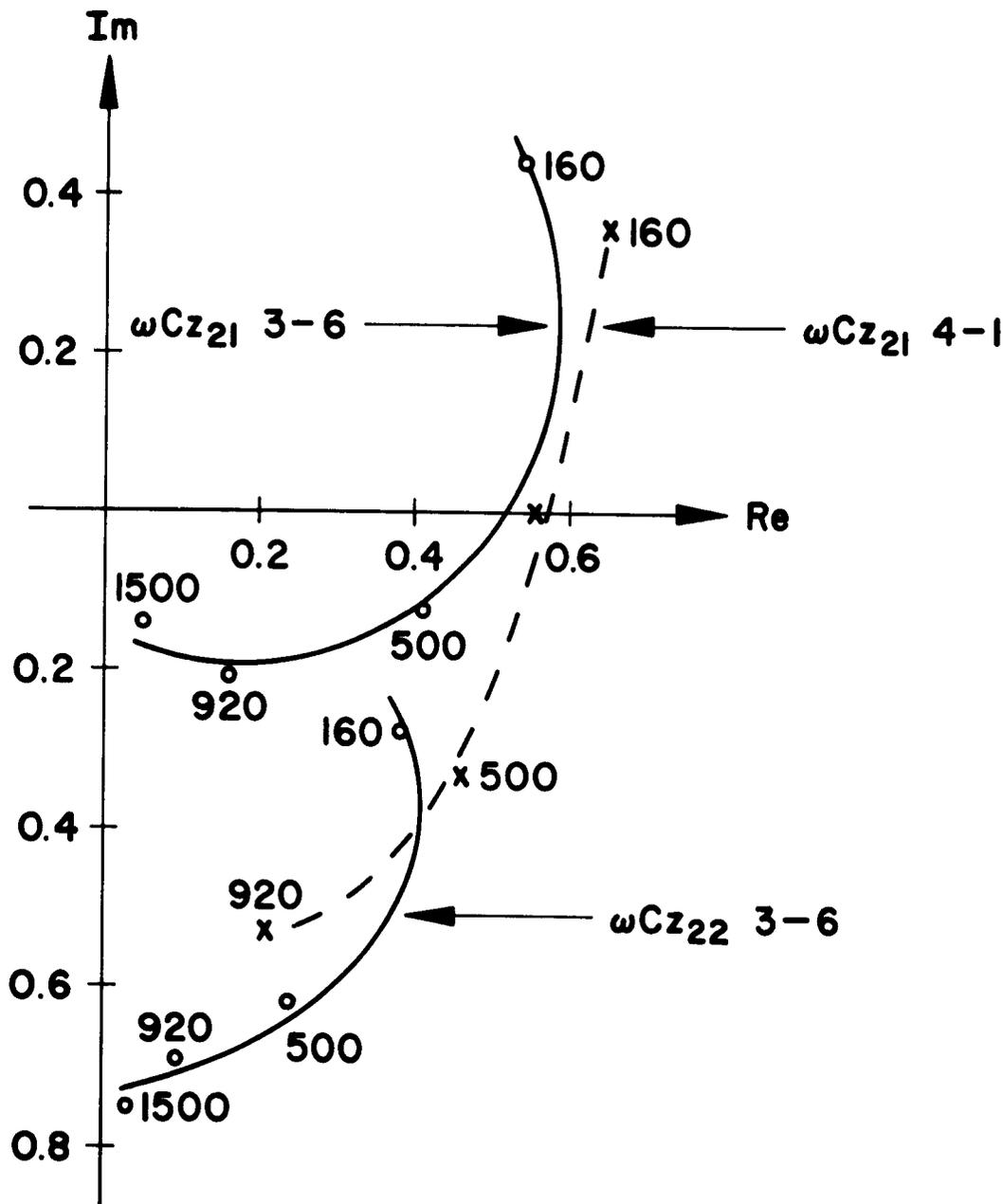
Fig. 5. Real and imaginary parts of  $\omega C Z$  with frequency in  $M_c$  as a parameter
