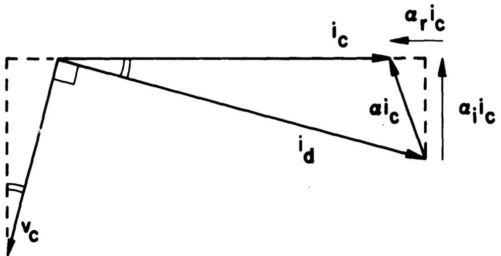
Fig. 2. Phasor diagram of currents
