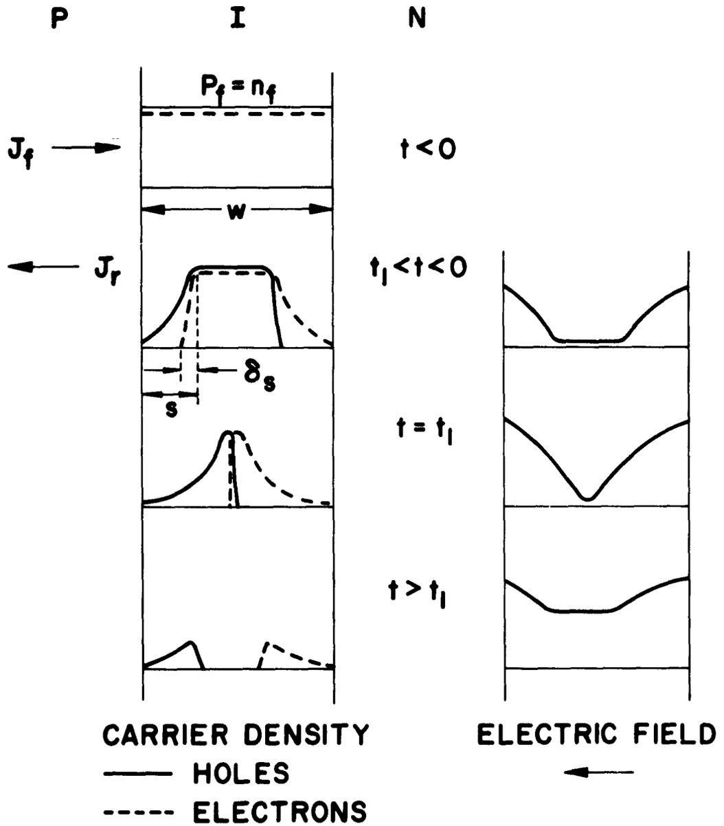
Fig. 6. Transient PIN carrier densities and electric field
