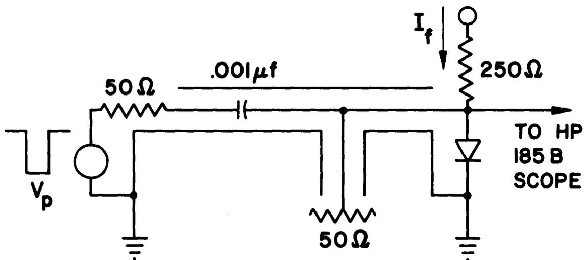
Fig. 9. PIN diode transition time test circuit.
