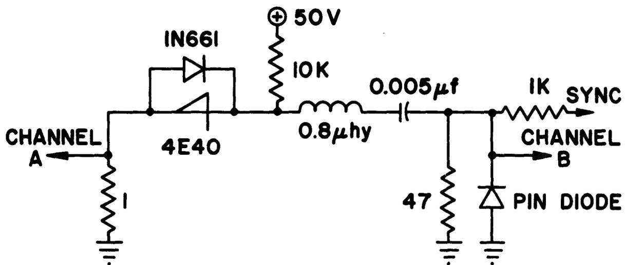
Fig. 8. PIN diode lifetime test circuit
