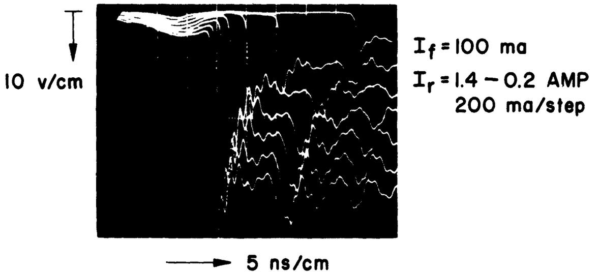
Fig. 10. Small-area diode storage and transition times
