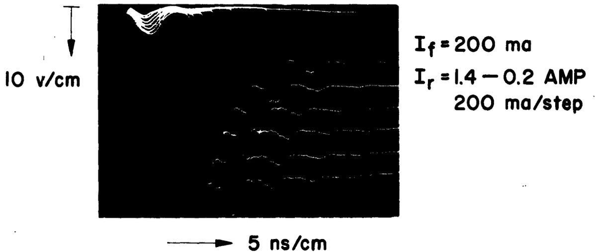
Fig. 11. Large-area diode storage and transition times
