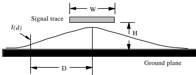
**Figure 4. Current density distribution (trace to reference plane)**
