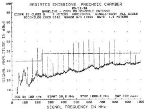
**Figure 5. Baseline measurement of radiated emissions**
