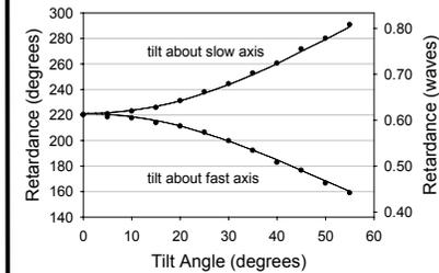
780nm half-wave plate tilted about the fast and slow axis. 637.5nm laser used. Solid curves show results of Hinds PEM. Dots show result of our gelatin PEM.
