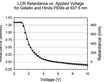
We used the gelatin PEM to measure the optical activity of a glucose solution, with concentrations varying between 0 and 100 g/L. The line is from the Hinds PEM and the black dots show the gelatin PEM results, indicating a close match between the two devices. A 637.5 nm laser was used for all measurements.
