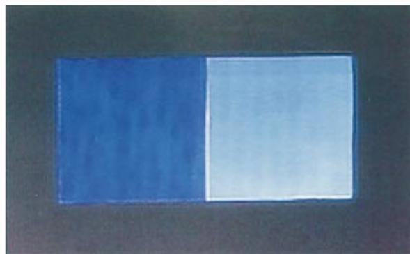
FIG. 6. (Color) Effectiveness of blocking the screen is compared between the cellophane sheet on the left and commercially available half-wave plate on the right.
