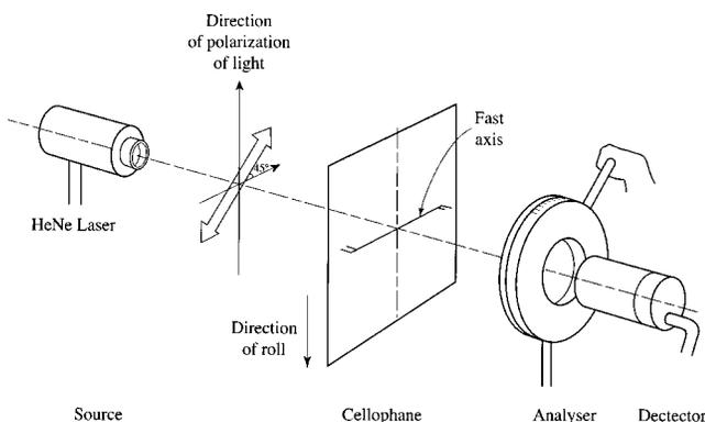
FIG. 2. Arrangement for measuring the retardance of cellophane.
