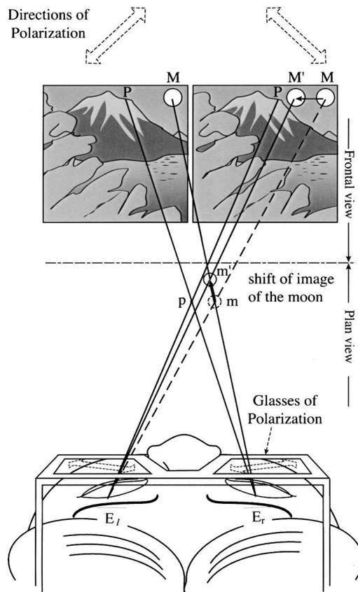
FIG. 7. Principle of the 3D display of the crisscross stereoscopic pair.
