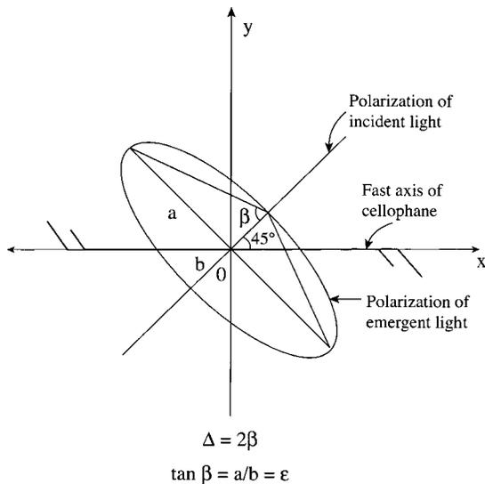
FIG. 1. Conversion of linearly polarized incident light to elliptically polarized light by a retarder.
