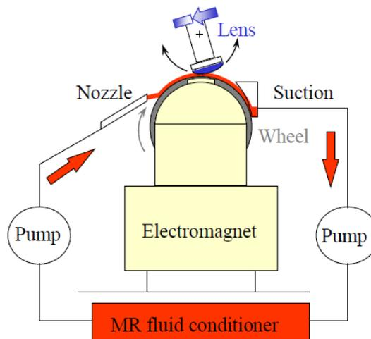
**Figure 5: Schematic of an MRF Machine**
