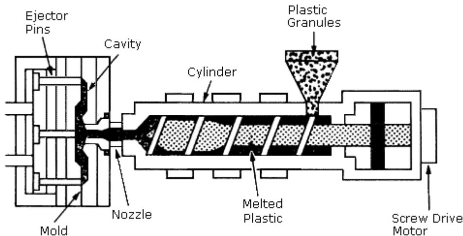
**Figure 10: Schematic of an injection molding tool**
