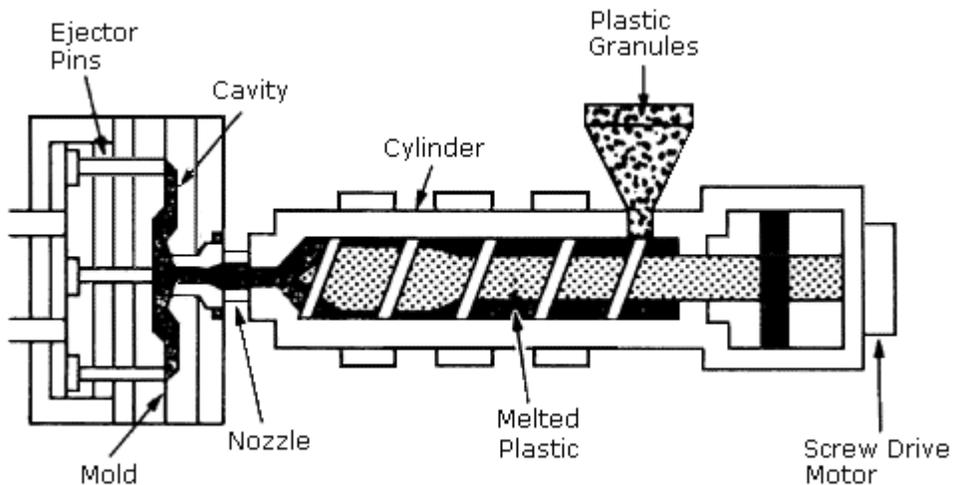
**Figure 10: Schematic of an injection molding tool**
