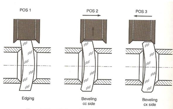
**Figure 7: Combination bevel and centering tool**
