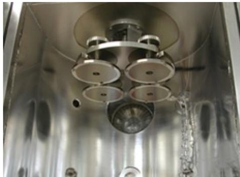
**Figure 8: Vacuum chamber and planetary optic holder**
