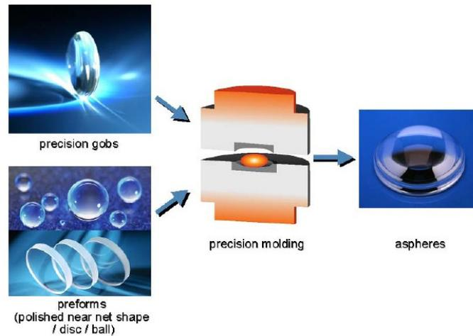
**Figure 9: Overview of the Molding Process (Schott)**
