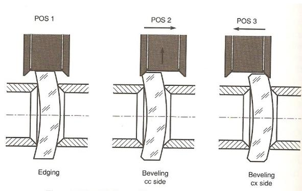
**Figure 7: Combination bevel and centering tool**
