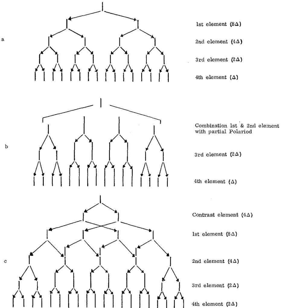
Fig. 4. Pulse response of 4-element Lyot filter (a), single partial polaroid filter (b), contrast element filter (c).
