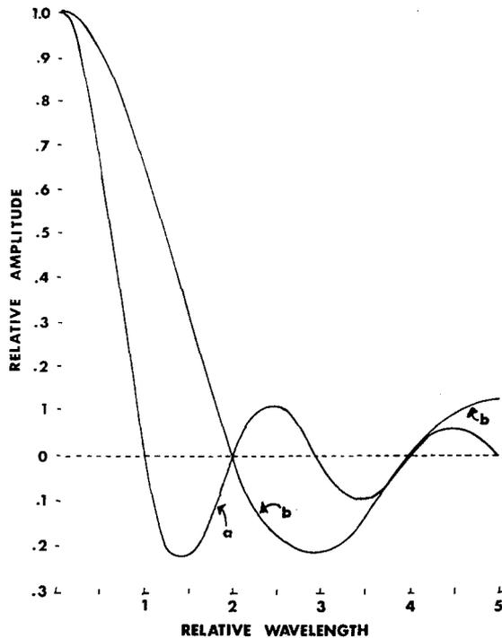
Fig. 2. Transmitted electric field intensity for a Lyot filter of length  $L$  (a) and  $L/2$  (b).
