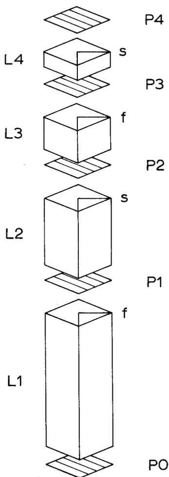
Fig. 1. Optical schematic of 4-element Lyot filter with alternate elements orthogonal.
