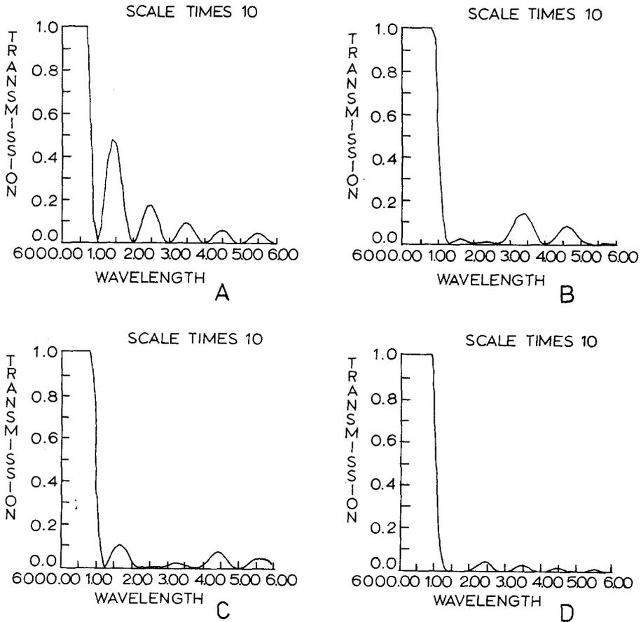
Fig. 3. Scale  $\times 10$  transmissions profile of normal Lyot filter (a), single partial polaroid filter (b), contrast element filter (c), two partial polaroid filter (d). All filters are of the same total length.
