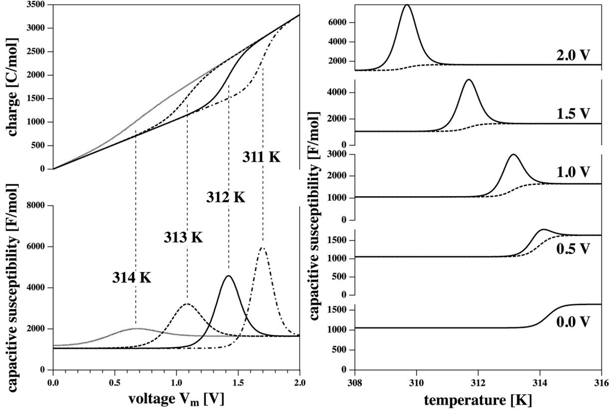
Figure 3: *Left: Voltage-induced transition of DPPC LUV at four different (constant) temperatures. Top panel: the charge as a functions of voltage. Bottom panel: capacitive susceptibility as a function of voltage. Right: Capacitive susceptibility  $\hat{C}_m$  as a function of temperature for five different voltages. The dashed lines represent the capacitance  $C_m$  as a function of temperature.*
