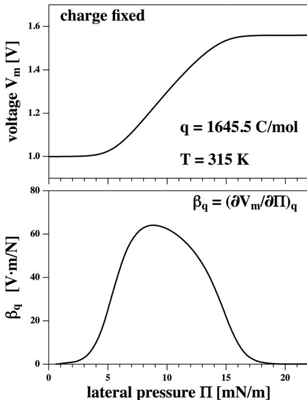
Figure 5: *Top: Change in voltage induced by lateral pressure changes at fixed charge on the capacitor ( $C_m=1430.7$  C/mol corresponding to the charge on the fluid phase membrane at  $V_m=1$  V). Increasing lateral pressure renders the membrane more solid. Bottom: The corresponding susceptibility,  $\beta_q = (\partial V_m/\partial \Pi)_q$ .*
