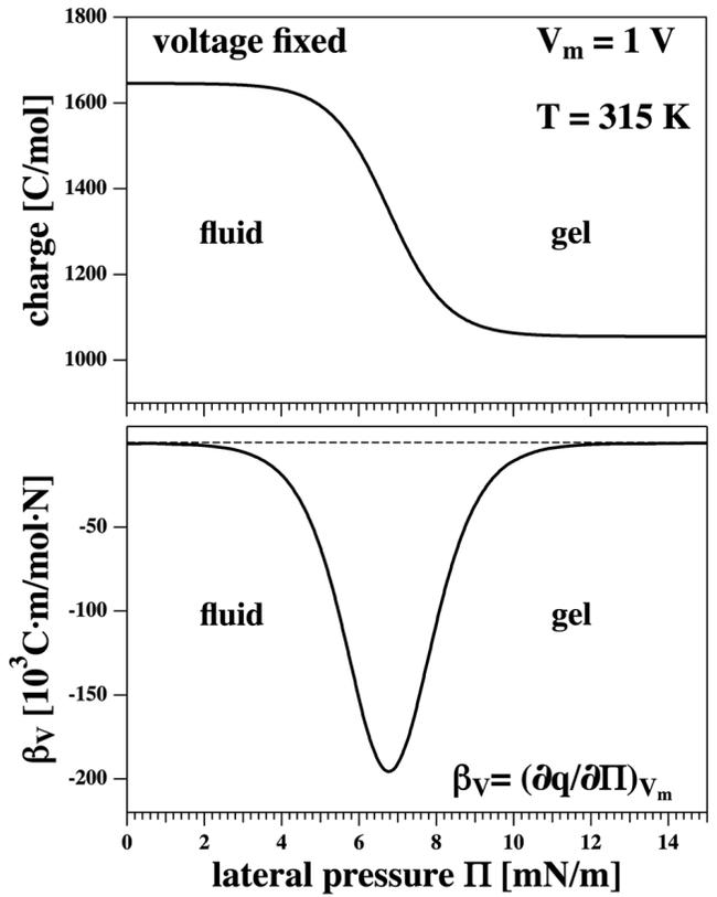
Figure 4: Changes in electrical properties induced by lateral pressure changes. Top: Change in the charge on a capacitor upon changes in lateral pressure at fixed voltage of  $V_m = 1 \text{ V}$ . Bottom: Change in voltage induced by lateral pressure changes at fixed charge on the capacitor ( $C_m = 1430.7 \text{ C/mol}$  corresponding to the charge on the fluid phase membrane at  $V_m = 1 \text{ V}$ ). Increasing lateral pressure renders the membrane more solid.
