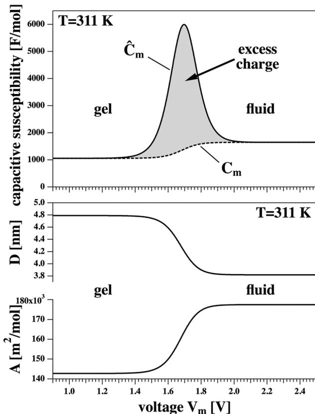
Figure 2: *Bottom: Area and thickness changes as a function of voltage at  $T = 311$  K. The temperature,  $T = 311$  K, is below the melting point of DPPC in the absence of voltage. Top: Capacitive susceptibility,  $\hat{C}_m$ , of DPPC LUV as a function of voltage. The shaded area indicates the excess charge of the voltage-induced transition. The dashed line is the voltage dependent capacitance,  $C_m$ .*
