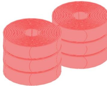
Fig. 2. Isometric, three layer double coil with bending angle  $0^\circ$ , inner diameter 8 mm, and outer diameter 30 mm. There is 0.1 mm space between the turns and 1 mm space between the layers.
