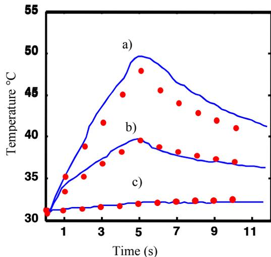
Figure 7. Temperature measured (- lines) and simulated (●) at 3 different locations located a) on the outer surface b) inside of the skull and c) on the inner surface.
