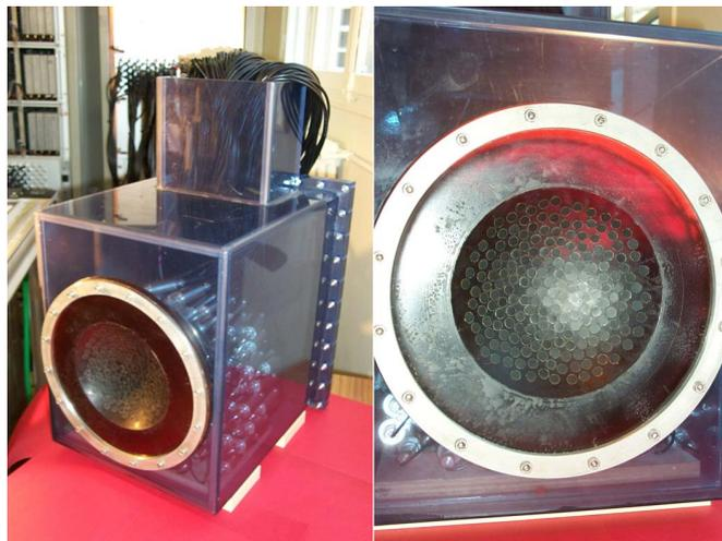
Figure 2. 200-Element high power ultrasonic array.
