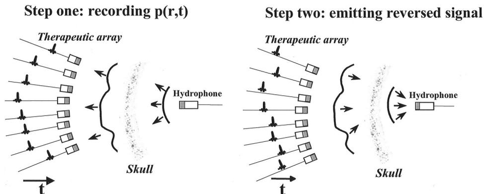
FIG. 3. Schematic of the time reversal correction. *Left:* First step. The wavefront emitted by the hydrophone is recorded on the therapeutic array after propagation through the skull. The equation  $p(r, t)$  represents pressure ( $p$ ) as a function of space ( $r$ ) and time ( $t$ ). *Right:* Second step. The time-reversed signals are reemitted and focused back to the initial location.
