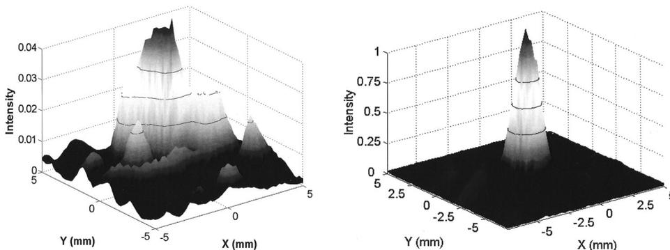
FIG. 4. Graphs showing the defocusing effect of the skull. The energy repartition in the focal plane is plotted in a linear scale without any correction (*left*) and with time-reversal correction (*right*).
