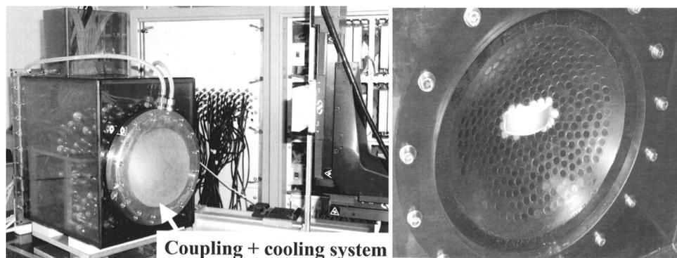
FIG. 1. Photographs showing a high-power time reversal prototype. *Left*: Large view of the high-power prototype with its cooling system. *Right*: Close-up view of the 277 therapeutic transducers mounted on a spherical surface. An echographic array has been inserted in the center of the array to guide the global positioning.
