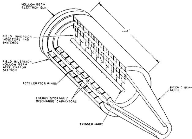
A one-MeV, one-ohm PULSITRON accelerator.
