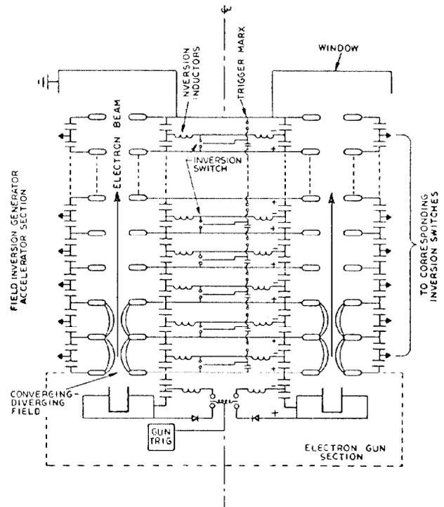
A schematic diagram of PULSITRON accelerator.
