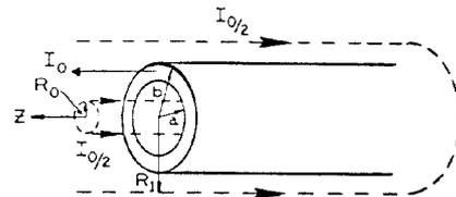
Hollow beam with equal inner and outer return currents.
