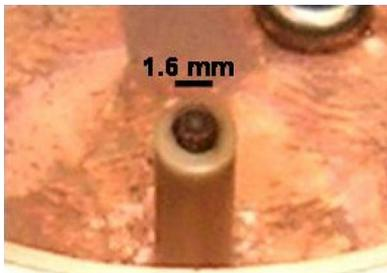
Fig. 3. Spot on the anode of the NF device after about thousand discharges. A spot is observed on the anode. The diameter of the anode is 1.6 mm, and the size of the spot is on the order of  $200 \mu\text{m}$ . The spot is probably due to the erosion produced by the electron beams impinging on the anode and by the interactions of the plasma pinch.
