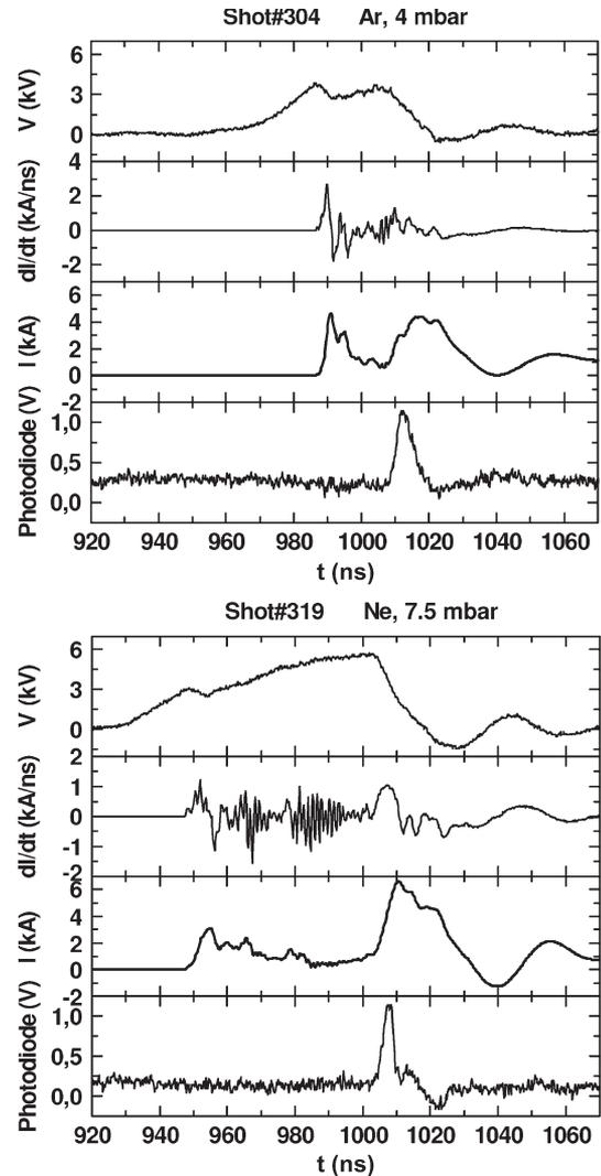
Fig. 4. Signals in an X-ray photodiode in correlation with the discharge for Ar and Ne.
