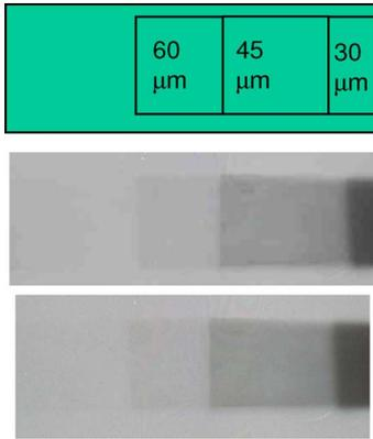
Fig. 2. Radiographs of an array of aluminum filters of 30-, 45-, and 60- $\mu\text{m}$  thickness on an HP5 Ilford film obtained after 1200 integrated shots of the NF operating at 0.4 Hz. Assuming a monoenergetic X-ray emission, an effective mean energy of  $4.3 \pm 0.3$  keV is estimated from the radiographs.
