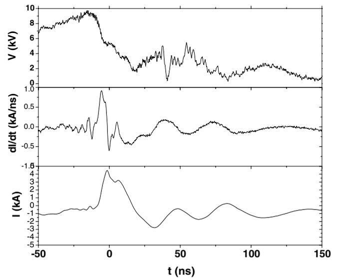
**Figure 6.** Electrical signals during a discharge in hydrogen at 3 mbar, with an initial charge of 9 kV (i.e. 0.2 J) using a 0.21 mm anode radius. A current peak of 4.5 kA was obtained. Evidence of a radial compression (pinch) is the dip observed in the current derivative signal (it is the frequency change in the  $dI/dt$  oscillation and has been used as time zero in the graph), coinciding with a drop in the electrical current.
