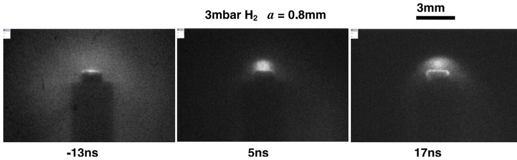
**Figure 5.** Sequence of photographs of the evolving plasma. The anode radius is  $a = 0.8$  mm. The following phenomena can be extracted from the observation of pictures: (a) the plasma is initiated over the insulator, (b) the plasma covers the anode, (c) there is a radial compression of the plasma over the anode, (d) finally the plasma separates from the anode in the axial direction. The time from stages (a) to (d) is about 30 ns.
