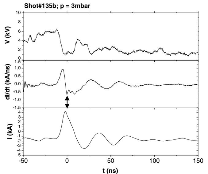
**Figure 4.** Electrical signals during a discharge in hydrogen at 3 mbar, with an initial charge of 6.5 kV (i.e. 0.1 J). The anode radius is  $a = 0.8$  mm. A current peak of 4.5 kA was obtained. Clear evidence that a radial compression (pinch) actually occurred is the dip observed in the current derivative signal (it is the frequency change in the  $dI/dt$  oscillation and has been used as time zero in the graph, indicated by the arrow), coinciding with a drop in the electrical current.
