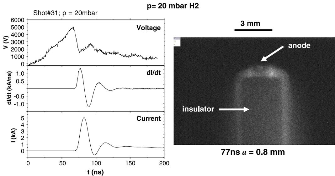
**Figure 3.** Electrical signals during a discharge in hydrogen at 20 mbar, with an initial charge of 5 kV. Also a photograph of the plasma at a later time of the discharge is shown. It can be seen that the plasma remains attached to the insulator, which is consistent with the behavior of PF discharges at high pressures.
