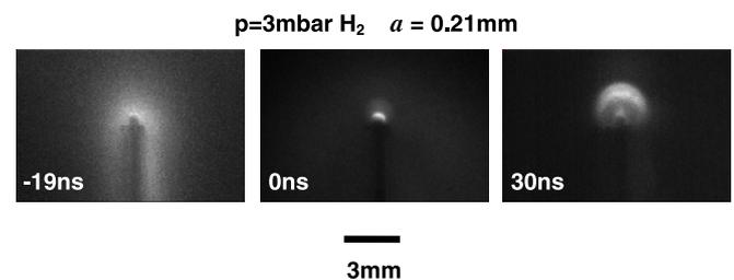
**Figure 7.** Sequence of photographs of the evolving plasma for discharges on anode radius  $a = 0.21$  mm. The plasma dynamics is similar to that observed in conventional PF discharges.
