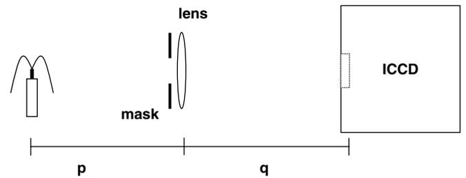
**Figure 2.** Optical system. For imaging the plasma over the microchannel plate in the ICCD camera, a regular bi-convex lens with 17.5 cm focal length and 5 cm diameter was used. A mask with an open circle of 0.8 cm diameter was attached to the lens in order to increase the field depth, resulting in an optical number  $F \cong 22$ . Value of other magnitudes:  $p = 35 \text{ cm}$ ,  $q = 35 \text{ cm}$ , magnification  $m = 1$ .
