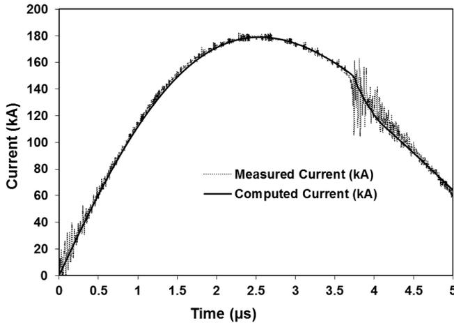
Fig. 2. Fitting of the measured current waveform (dotted line) with the computed current waveform (solid line) of UNU/ICTP PFF operated at 14 kV, 30  $\mu\text{F}$  and 2.8 Torr with neon gas.
