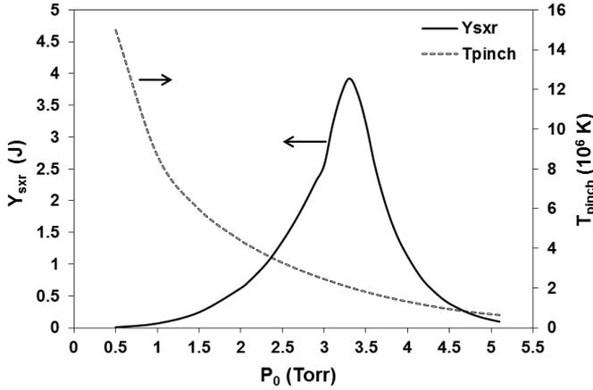
Fig. 3. Computed neon yields  $Y_{\text{sxr}}$  and the pinched plasma temperatures with respect to pressure of UNU/ICTP PFF operating at 14 kV and 30  $\mu\text{F}$ .
