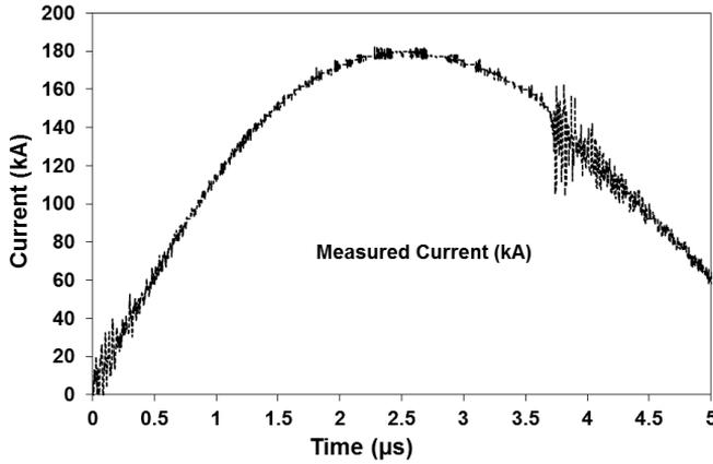
Fig. 1. Measured discharge current waveform of the UNU/ICTP PFF operated at 14 kV, 30  $\mu\text{F}$  and 2.8 Torr with neon gas.
