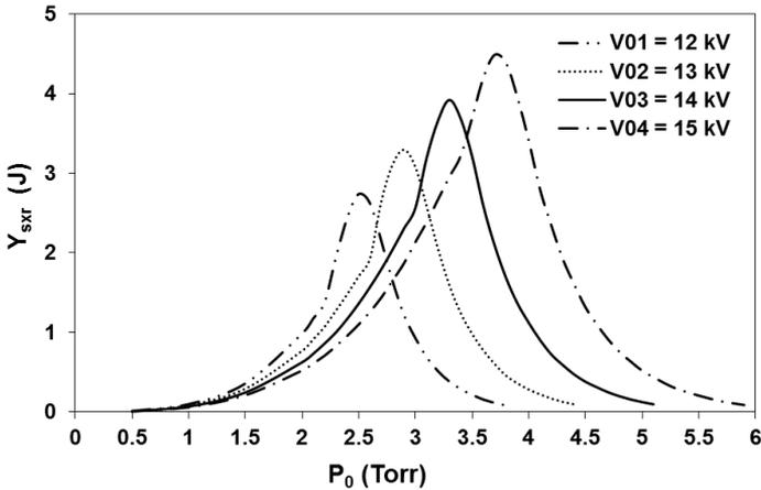
Fig. 4. Variations of computed neon yield  $Y_{\text{sxr}}$  from UNU/ICTP PFF versus pressure at different operating voltages.
