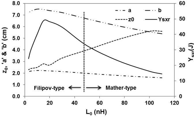
Fig. 6. Computed values of yield  $Y_{\text{sxr}}$  and its corresponding optimum electrode geometry with respect to  $L_0$  at 14 kV, 30  $\mu\text{F}$  and 2.0 Torr with neon gas.
