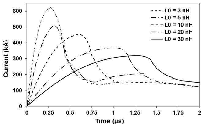
Fig. 5. Computed discharge current waveforms as a function of time for operation at 14 kV, 30  $\mu\text{F}$ ,  $P_0 = 3.3$  Torr of neon for operation with different values of  $L_0$ .
