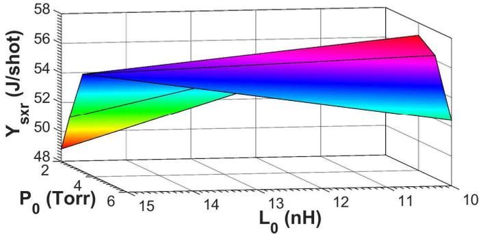
Fig. 7. A 3D plot of optimum neon  $Y_{\text{sxr}}$  versus optimum  $L_0$  at six operating  $P_0$  for our optimization at 14 kV and 30  $\mu\text{F}$ .
