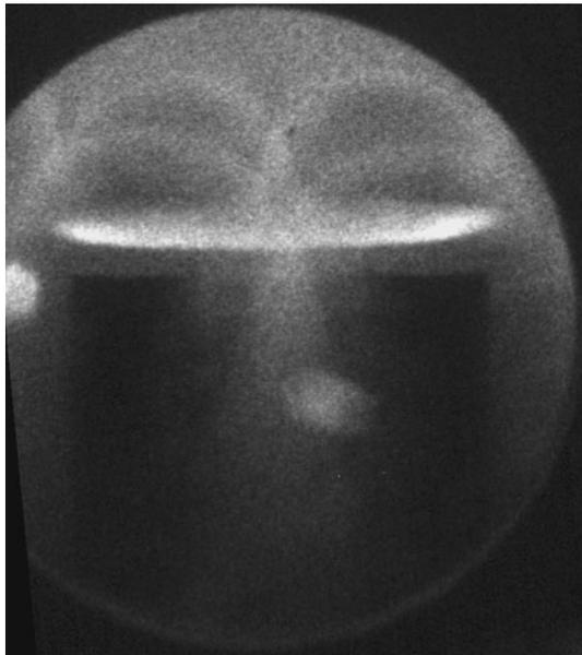
**Fig. 5** ICCD image of end of anode at 225 ns before pinch, exposure time 0.2 ns. Note the convergence of the filaments at this time on the axis of the anode. The *circle* is the viewing window and the *bright horizontal ellipse* is the hole in the anode
