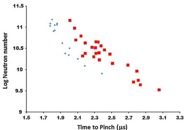
**Fig. 2** Log neutron yield vs time to pinch. The *small dots* are shots at 10 torr fill pressure while the *large ones* are at 18–24 torr. Error bars are omitted for clarity and are 0.1 for log yield and extremely small—less than 5 ns—for time. Quarter-cycle time is 1.8  $\mu\text{s}$
