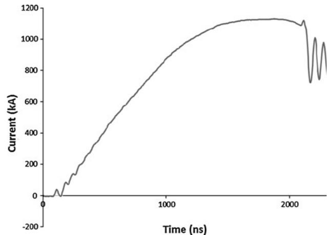
**Fig. 3** Current vs time, shot 10011002, an LPT, with pinch process starting with negative  $dI/dt$ . Note the small bump in current before the pinch
