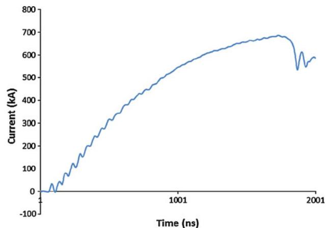
**Fig. 4** Current vs time, shot 03301010, a SPT with pinch process starting with positive  $dI/dt$ . Note the smooth decline in current into the pinch
