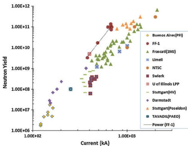
**Fig. 6** FF-1 SPT results, *filled circles on line*, fall above the historic trend line of DPF results. Data is from M. Milanese and J. Pouzo [31], except for U of Illinois and FF-1. *Line* is power-law fit to FF-1 data
