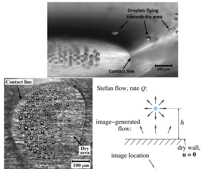
FIG. 2. Photos of levitating water droplets: (top) Side view of droplet fly-over near the contact line at  $T_w = 90^\circ\text{C}$ ; (bottom left) array of droplets over the dry patch viewed from the top at  $T_w = 85^\circ\text{C}$ ; (bottom right) sketch for the derivation of levitation condition. See also videos S3 and S4 in the Supplemental Material [15].
