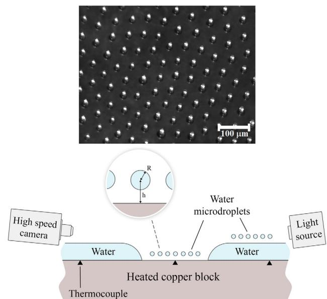
FIG. 1. (top) Array of levitating droplets over the liquid-gas interface viewed from the top. (bottom) Sketch of the experimental setup used for studies of droplet arrays over both liquid surface and dry substrate; droplet radius  $R$  and levitation height  $h$  are shown.
