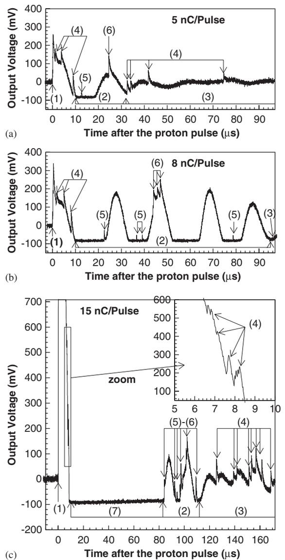
Fig. 1. Waveforms (output voltage as a function of time) recorded after one proton pulse with a  $^{235}\text{U}$  coated solar cell (without compensation) in the LSDS, for 3 different proton pulse sizes: 5 nC (a), 8 nC (b) and 15 nC (c). Time 0 corresponds to the incident proton pulse. Fission signals are indicated by arrows (see text for additional discussion).
