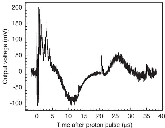
Fig. 4. Waveform obtained in the LSDS with the compensated setup in the case of a 40 nC proton pulse (preamplifier output). The amplitude of the excursions near  $t = 0$  is drastically reduced compared to Fig. 1(c) and fission signals are observed.
