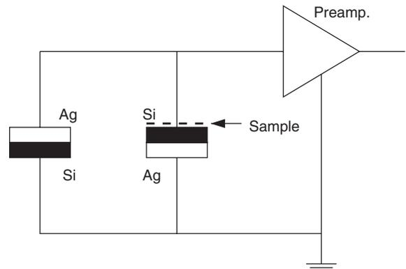
Fig. 2. Diagram of the compensated fission detector. The cells are connected in antiparallel order to compensate (by subtraction) the signals induced by the  $\gamma$ -flash.
