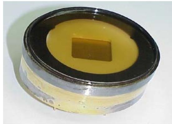
**Figure 15.** A photograph of a sealed GEM- gaseous detector with a semitransparent K-Cs-Sb photocathode.
