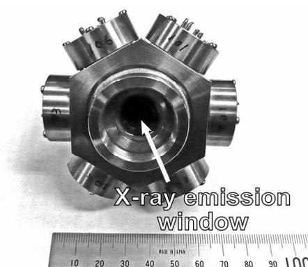
**Figure 1.** Photograph of the X-ray source.
