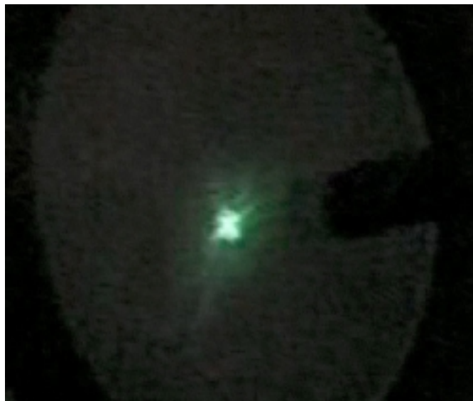
Fig. 23 Photograph of the electron beam image as the pressure rises through about 3mTorr and the beam begin to defocus and become unstable
