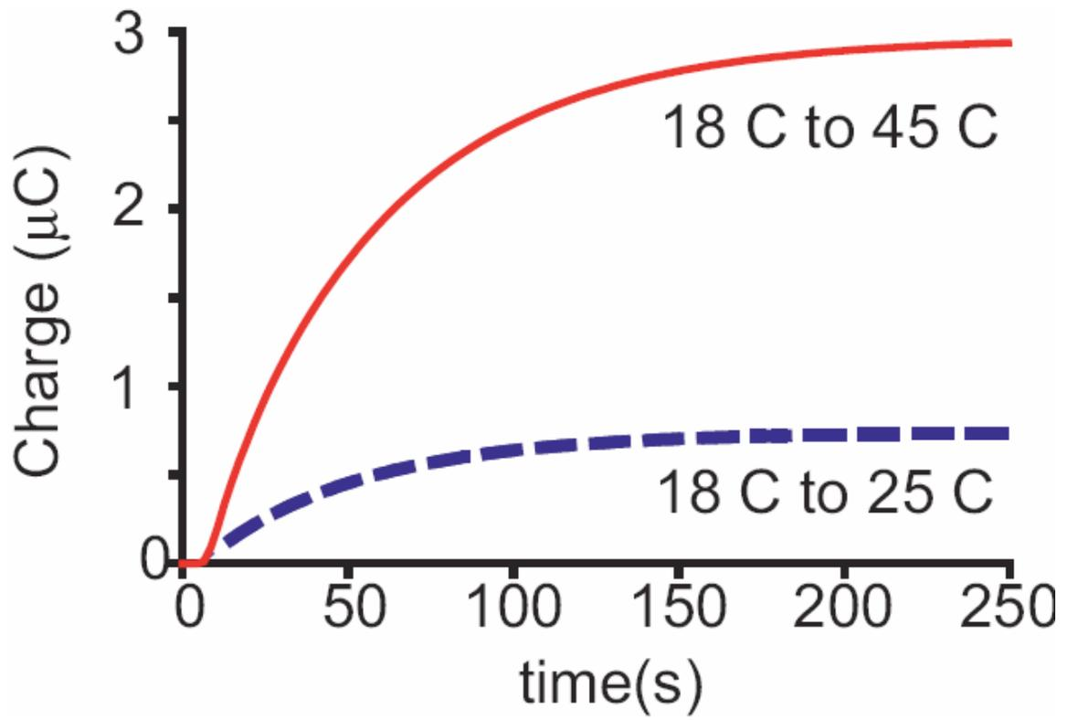
Figure 3) Direct charge measurements in air (1 atm) for different temperature ramps.
