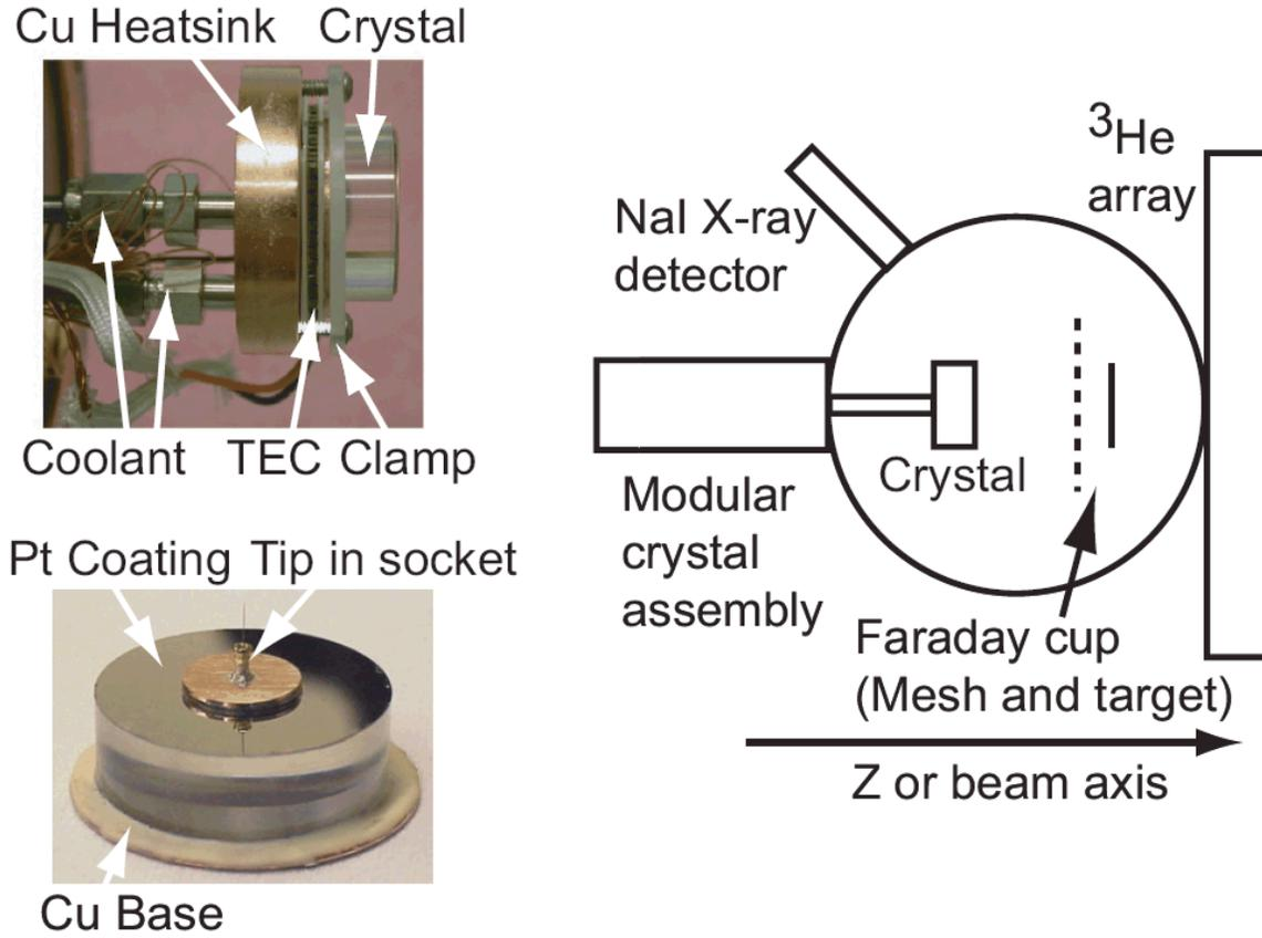
Figure 2) Schematic of the CDNS with close-up views of the modular crystal assembly and one of the crystals. The crystal can be moved back and forward along the beam axis. The thermocouple for feedback control is sandwiched between the TEC and the copper backplate on the rear of the crystal. A groove cut into the backplate allows the thermocouple to be sandwiched snugly without causing a gap between the TEC and the backplate.
