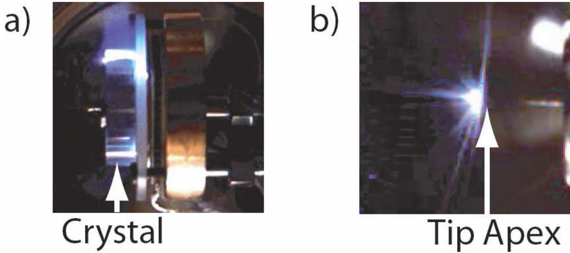
Figure 6a) Typical surface flashover breakdown on crystal side. 6b) Arcing to field emitter tip; the 0.02" diameter shank is visible but the tungsten tip and its apex is not due to its small radius. The socket mount design shown here is slightly different than the one described in Section II.
