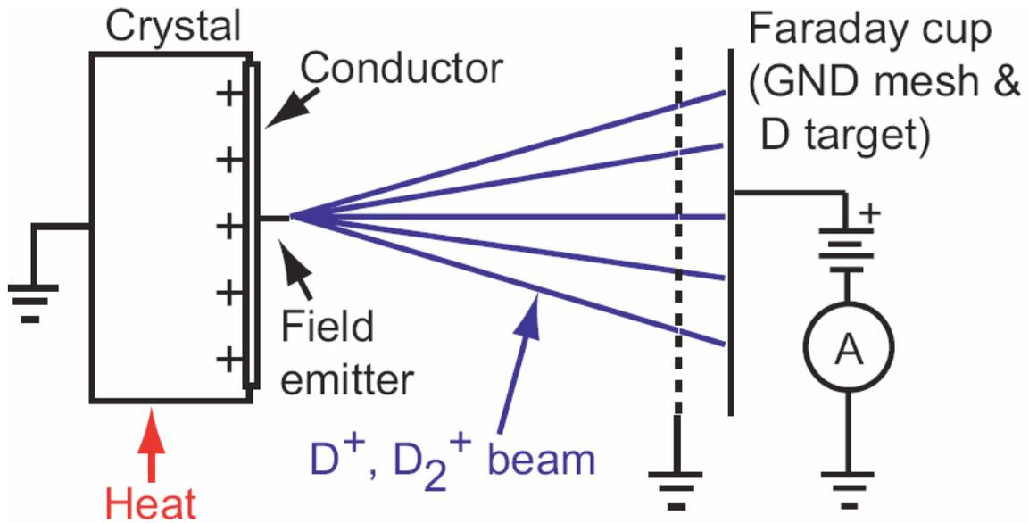
Figure 1) Schematic of the pyrofusion concept and a typical Faraday cup-target setup for ion current measurement [1]. The current collector or target plate behind the grounded mesh is loaded with deuterium for D-D fusion and connected to an ammeter for current measurement. The collector is operated with a positive bias to prevent the escape of secondary electrons [7].
