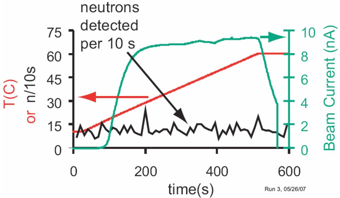
Figure 5) Measured beam current (right), detected neutrons per 10 s (left), and rear crystal temperature (left) for highest measured current run. The beam energy was only ~35-40 keV. The beam collapsed at ~575 s due to breakdown. Very few neutrons above background were detected for this run due to the low beam energy.
