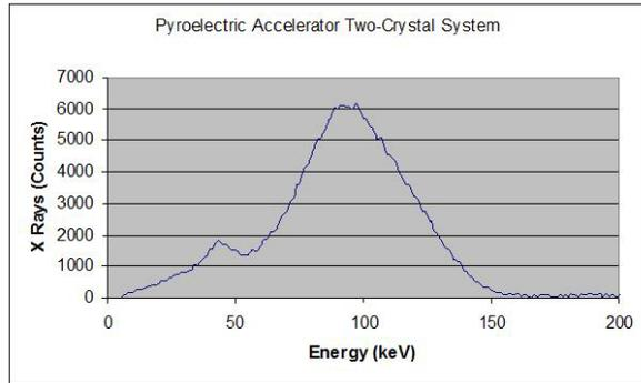
**FIGURE 3.** A graph of a Bremsstrahlung x-ray spectrum generated by the field ionization and acceleration of residual gas particles from a two-crystal system inside a vacuum chamber over a 5 minute counting period. The end-point energy indicates an acceleration potential of approximately 150 keV. The lower energy x-rays may have been absorbed or scattered by the stainless steel vacuum chamber wall. A 5 minute background radiation spectrum was stripped out of these results.
