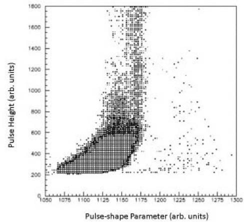
FIGURE 5 TWO-DIMENSIONAL PRESENTATION OF NEUTRON DETECTOR PULSE HEIGHT VERSUS PULSE-SHAPE PARAMETER. THE INTENSE BAND OF EVENTS TO THE LEFT OF CHANNEL 1190 IS DUE TO PILE-UP X-RAY EVENTS AND ENVIRONMENTAL GAMMA-RAY BACKGROUND, WHILE THE EVENTS TO THE RIGHT ARE DUE TO NEUTRONS FROM THE  $^3\text{H}(d,n)^4\text{He}$  REACTION
