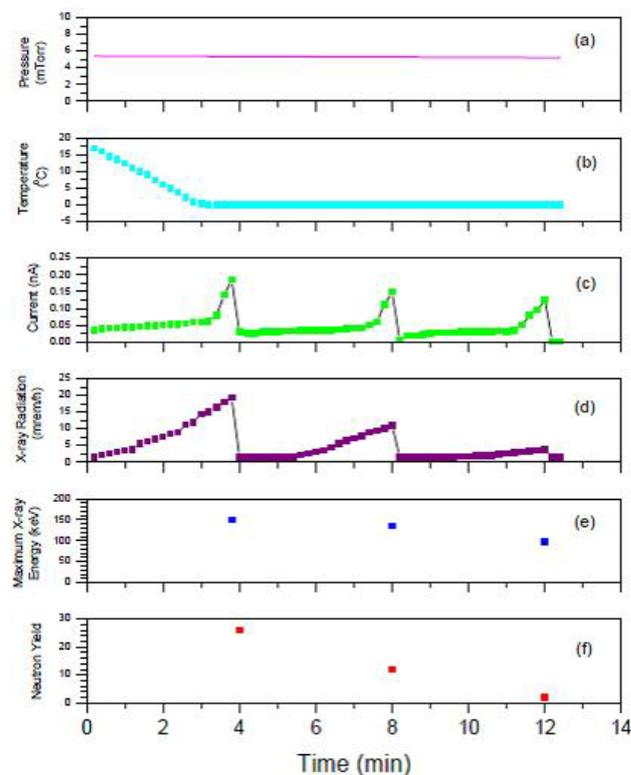
FIGURE 3 PARAMETERS MONITORED DURING COOL-DOWN PHASE OF PYROELECTRIC CRYSTALS AS FUNCTION OF TIME FOR A RUN IN THE EARLY STAGE OF OUR MEASUREMENTS: (a) PRESSURE, (b) TEMPERATURE, (c) CURRENT MEASURED ON THE DISK SHOWN IN FIGURE 1, (d) RADIATION LEVEL MEASURED WITH GEIGER COUNTER SHOWN IN FIGURE 1, (e) MAXIMUM X-RAY ENERGY RECORDED WITH HPGe DETECTOR SHOWN IN FIGURE 1, AND (f) NEUTRON YIELD ABOVE BACKGROUND OBTAINED BETWEEN DISCHARGES (SEE TEXT)
