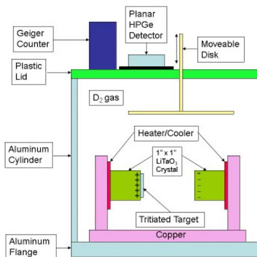
FIGURE 1 SCHEMATIC OF DOUBLE-CRYSTAL ARRANGEMENT WITH TRITIATED TARGET ATTACHED TO THE  $\text{LiTaO}_3$  CRYSTAL TO THE LEFT, AND GEIGER COUNTER AND HIGH-PURITY GERMANIUM (HPGE) DETECTOR PLACED ON TOP OF THE CHAMBER
