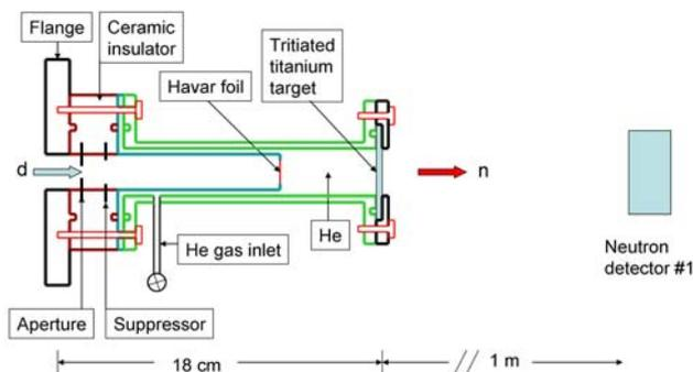
FIGURE 7 TARGET CELL USED TO PRODUCE  ${}^3\text{H}(d,n){}^4\text{He}$  NEUTRONS WITH TANDEM VAN DE GRAAFF ACCELERATOR, AND LOCATION OF NEUTRON DETECTOR #1. THE DEUTERON BEAM ENTERING ON THE LEFT SIDE IS PRODUCED BY TUNL'S TANDEM VAN DE GRAAFF ACCELERATOR
