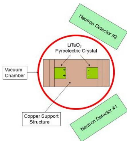
FIGURE 2 SCHEMATIC OF TOP VIEW OF CHAMBER SHOWN IN FIGURE 1, INDICATING THE LOCATION OF THE TWO NEUTRON DETECTORS
