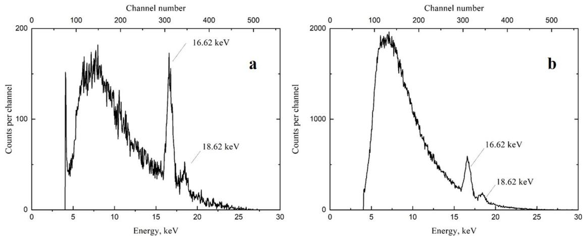
**Figure 2.** The spectra of X-ray radiation measured in quasi-continuous mode at the heating of the pyroelectric crystal from 25°C to 75°C during 300 s (a), and in pulsed mode after turning on the filament at 75°C during 5 seconds (b).
