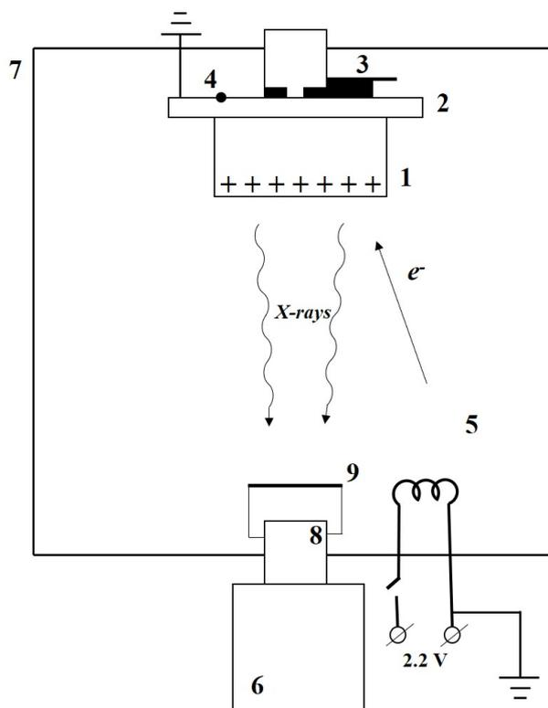
**Figure 1.** The experimental setup. 1 — pyroelectric crystal  $\text{LiNbO}_3$ , 2 — aluminum heat-conductor, 3 — silicon diode MUR 1560, 4 — thermocouple K type, 5 — filament, 6 — semiconductor X-Ray detector, 7 — vacuum chamber, 8 — entrance Beryllium window of the X-ray detector, 9 — maylar foil installed in front of the entrance window of the detector.
