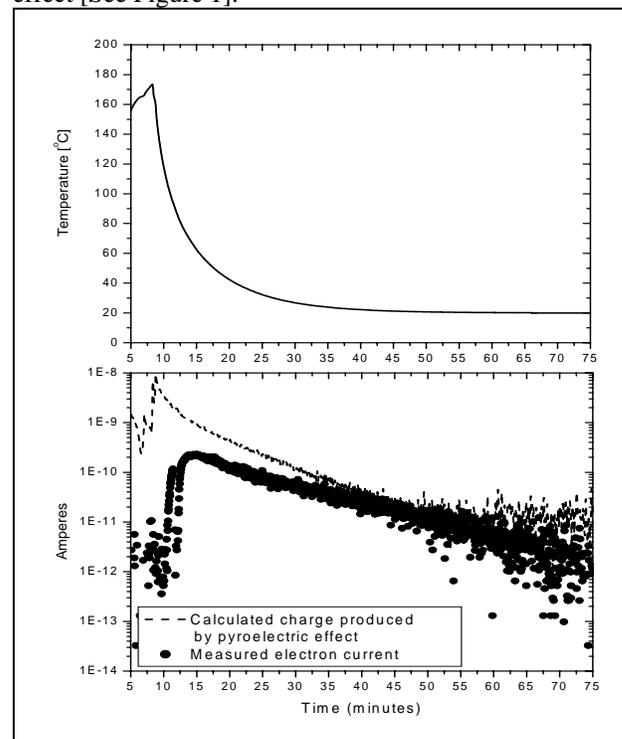
**Figure 1** - Electron current transmitted through 1-mil Be window as a function of time versus charge created due to the pyroelectric effect and temperature.
