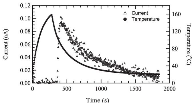
**FIG. 2.** Current and temperature as a function of time for a 1-cm  $\times$  0.5-cm lithium tantalate crystal. Temperature was measured at the grounded surface of the crystal; the temperature at the exposed surface of the crystal would be lower.
