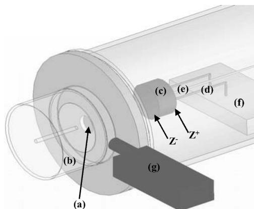
**FIG. 1.** Drawing of the experimental apparatus used to measure pyroelectric electron emission current and energy. (a) beryllium window, (b) Faraday cup, (c) pyroelectric crystal, (d) heating resistor leads, (e) thermocouple, (f) aluminum base, (g) X-ray detector.
