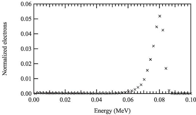
**FIG. 5.** Energy spectrum of the electrons incident upon the surface of the skin calculated using MCNP. Values are normalized for one source electron.
