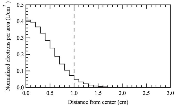
**FIG. 6.** Radial distribution of the electron flux incident upon the surface of the skin calculated using MCNP. Values are normalized for one source electron. The dashed line indicated the boundary of the treatment volume.
