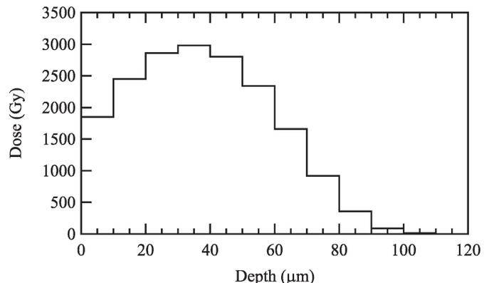
**FIG. 7.** Dose as a function of depth as delivered to  $10\text{-}\mu\text{m}$ -thick slices calculated using MCNP with  $3.77 \times 10^{12}$  incident electrons.
