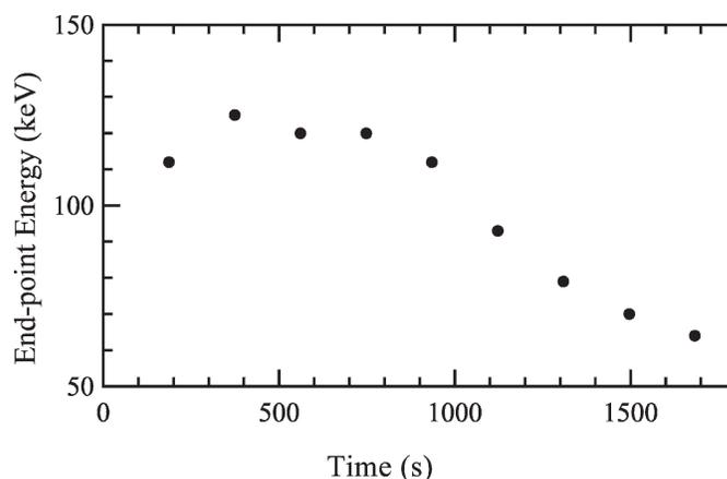
**FIG. 3.** Electron energy measured from the end point of the X-ray spectrum resulting from interactions of the electrons with the copper Faraday cup for the 1-cm  $\times$  0.5-cm lithium tantalate crystal. For this arrangement, Eq. (2) predicts a potential of 596 kV (assuming  $\Delta T = 140^\circ\text{C}$ ).
