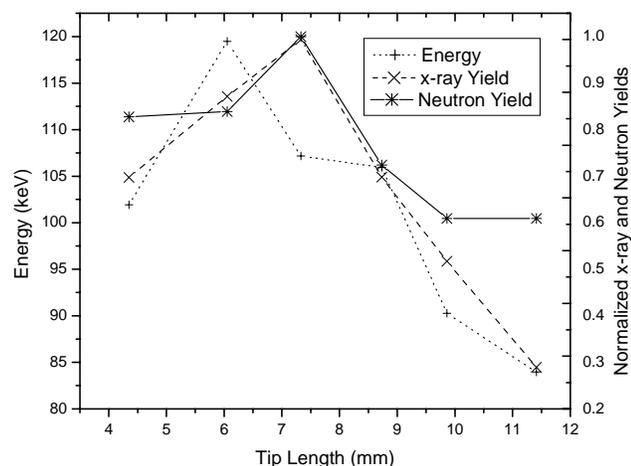
Fig.3. X-ray energy and yield versus tip length.
