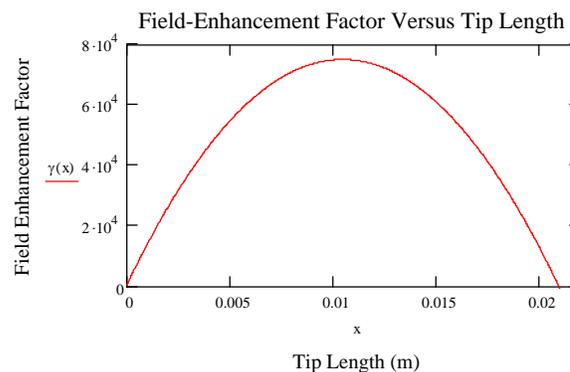
Fig. 1 Calculated tip length optimum
