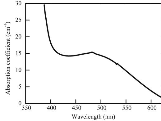
FIG. 4. Absorption spectrum of Fe-doped LN coated with ITO.
