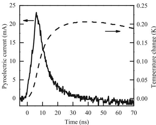
FIG. 3. Time dependence of pyroelectric current and calculated temperature change.
