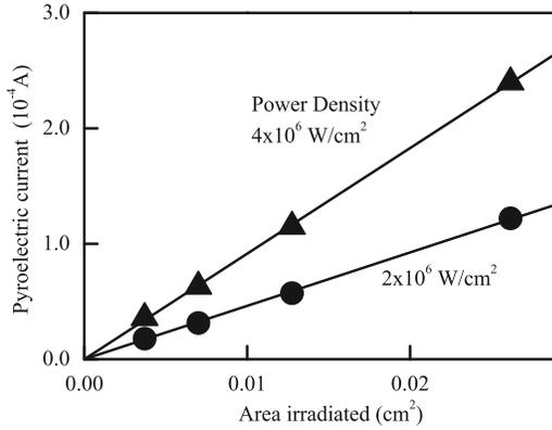
FIG. 2. Dependence of pyroelectric current  $I_{\text{pyro}}$  on beam area for two different power densities.
