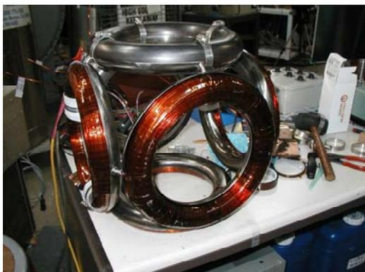
**Figure 11.** Construction detail of WB-6 coils
