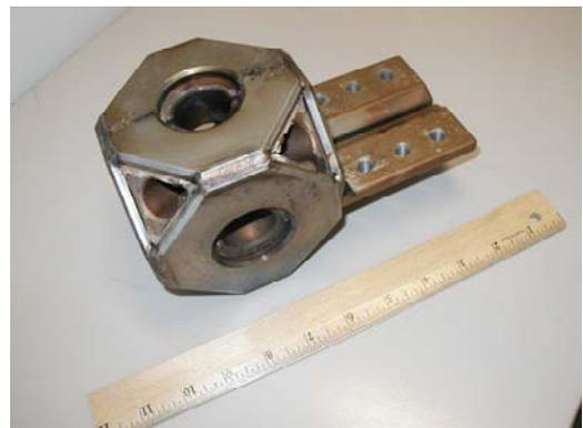
**Figure 9.** Pulsed compression device PZLx-1 built to study hydromagnetic stability of polyhedral field
