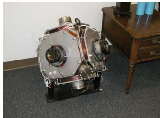
**Figure 8.** PXL-1 reactor for studying the electron cyclotron resonance
