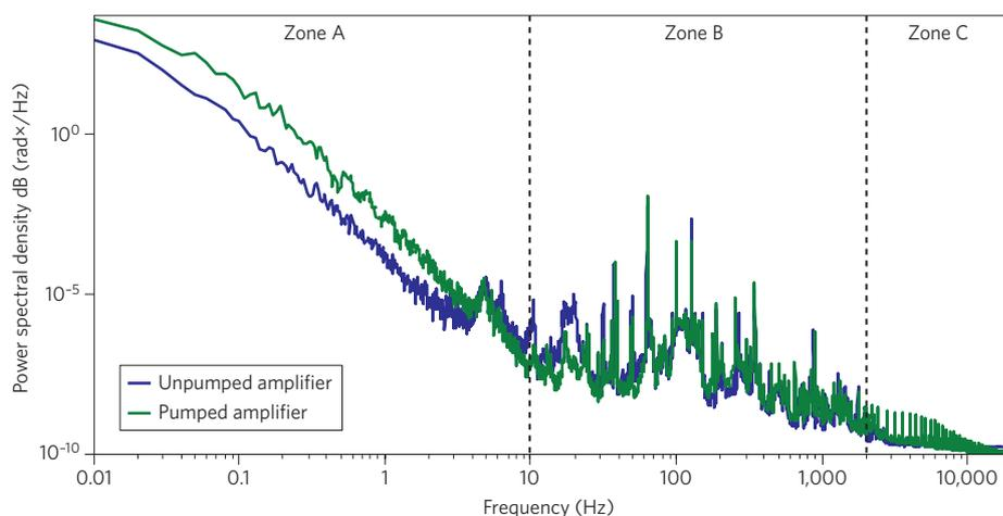
**Figure 2** | Phase noise spectra of a fibre amplifier unpumped (thin line) and pumped (thick line). In zone A phase noise mostly originates from thermal noise, in zone B from acoustic noise and in zone C from electrical noise. Most of the phase noise is thermal (zone A), and can be corrected with slow feedback loops if acoustic noise (zone B) is reduced passively (data from L. Lombard and G. Canat, ONERA).
