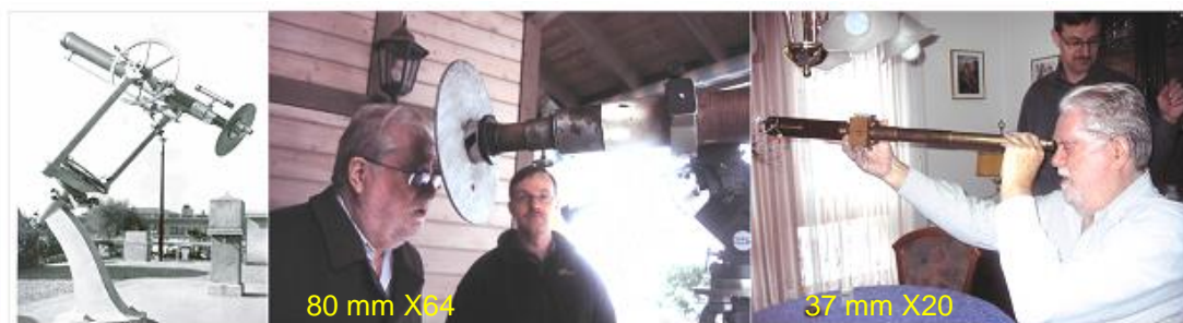
Figure 4. (Left) the 80 mm Fraunhofer refractor used since 1855 by Wolf and successors. (Center) the same telescope in use today by Thomas Friedli (person at right). (Right) the 37 mm portable telescope used by Wolf since the mid 1860s.
