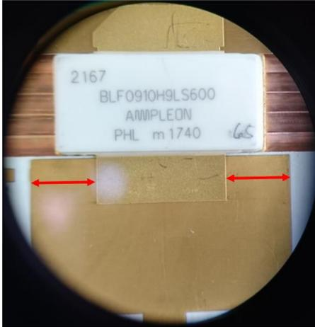
**Figure 4. The transistor should be centered inside the matching networks. Both arrows indicate the same distance from lead to edge matching network**
